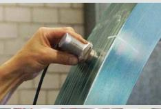
Surface crack testing
